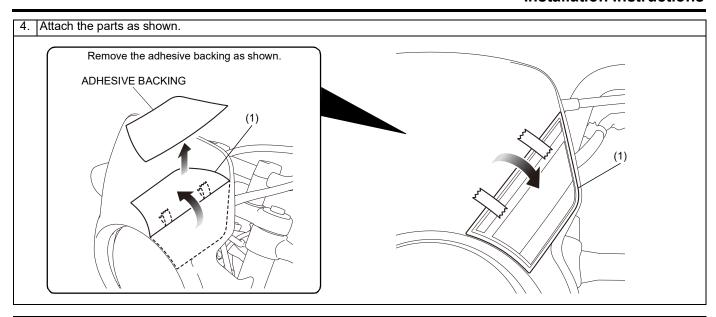
5. Apply adequate pressure to the attached parts.
